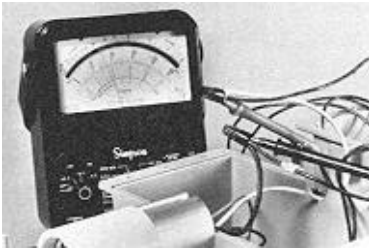
Open Circuit Voltage rest at Socket Head Connection
