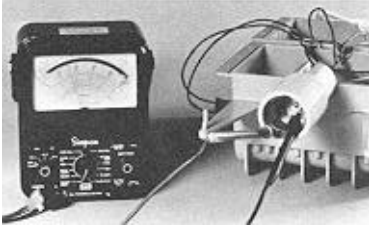
Open Circuit Voltage rest at Socket
