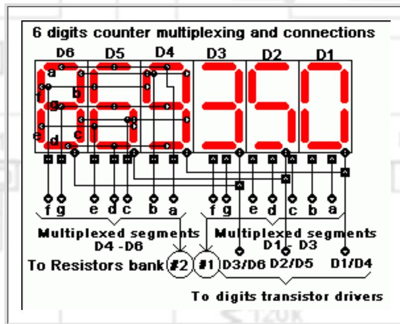
Example of single ( with jumpers in red ) or double layer PCB for six digits , size .56" common anode , standard pin layout .
