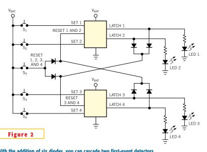
With the addition of six diodes, you can cascade two first-event detectors.
