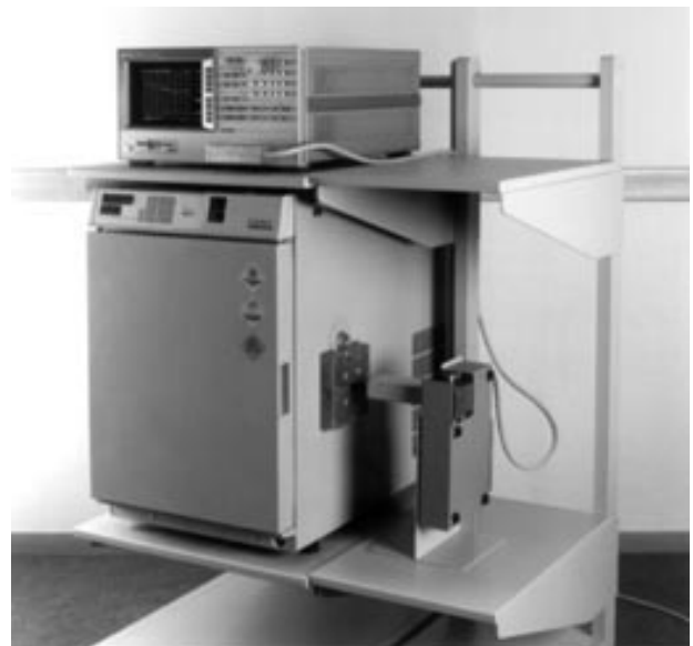
Figure 10. Configuring a system using the Tabai Espec SU-240-Y temperature chamber
