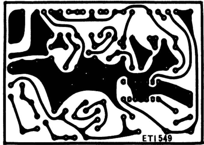
Fig.3 The PCB pattern. Most components other than the meter circuitry is built on this.
