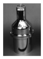
Bicron *Multiline* detector assemblies are scintillator-photomultiplier combinations that allow the removal of the photomultiplier tube or tubes without disturbing the scintillator package. The scintillator is mounted with appropriate reflector material in a low-mass metal container that has a glass or quartz optical window for each PMT. The magnetic light shield of each PMT is mechanically fastened to the flange or other mounting hardware on the scintillator container.
