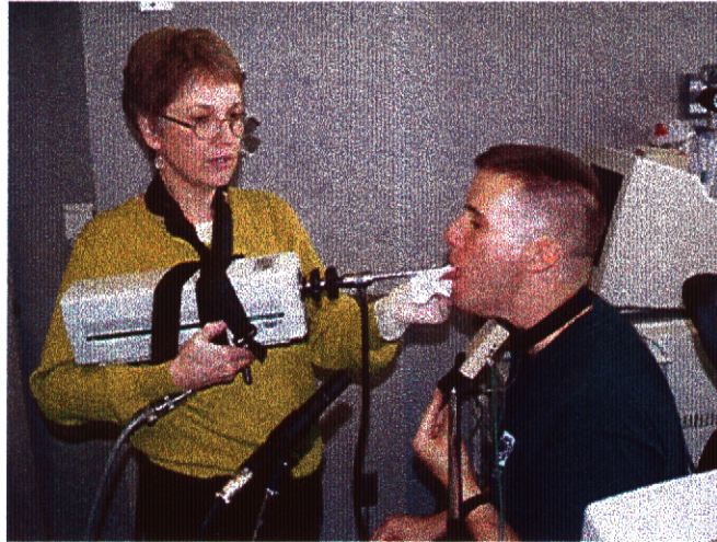
Figure 9 Gathering data with a laryngoscope coupled to a high speed digital movie camera, an EGG, the MIR speech sensor, and a microphone at the UC Davis medical center.
