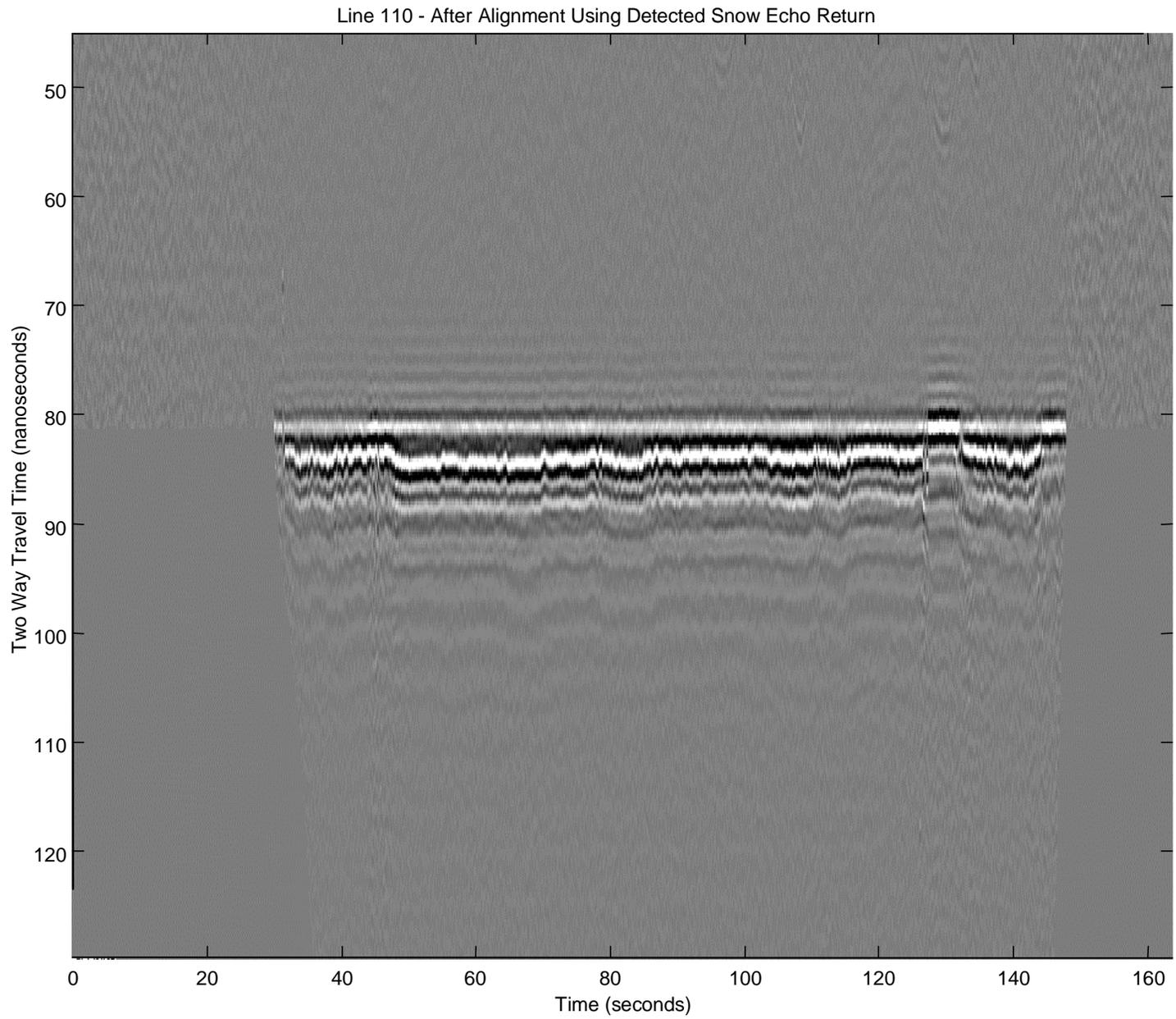
Figure 7. Analog data after aligning the radar returns using the air/ice interface echo.
