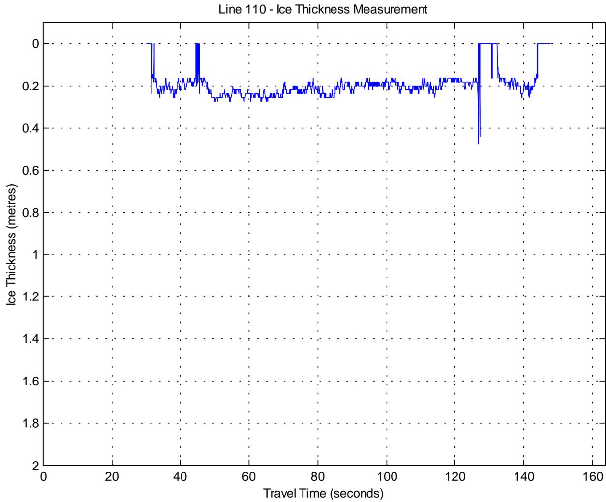
Figure 8 . Plot of fresh water ice thickness measurement using analog data.
