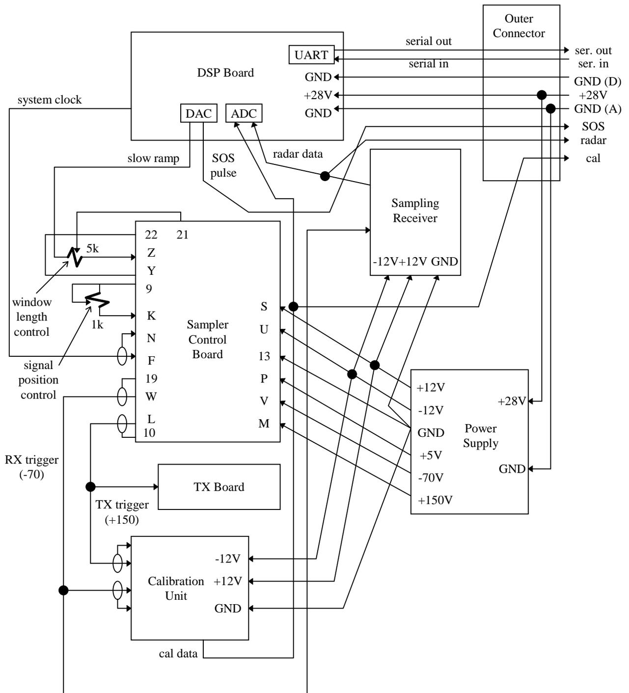
Figure 2. Wiring diagram of major components
