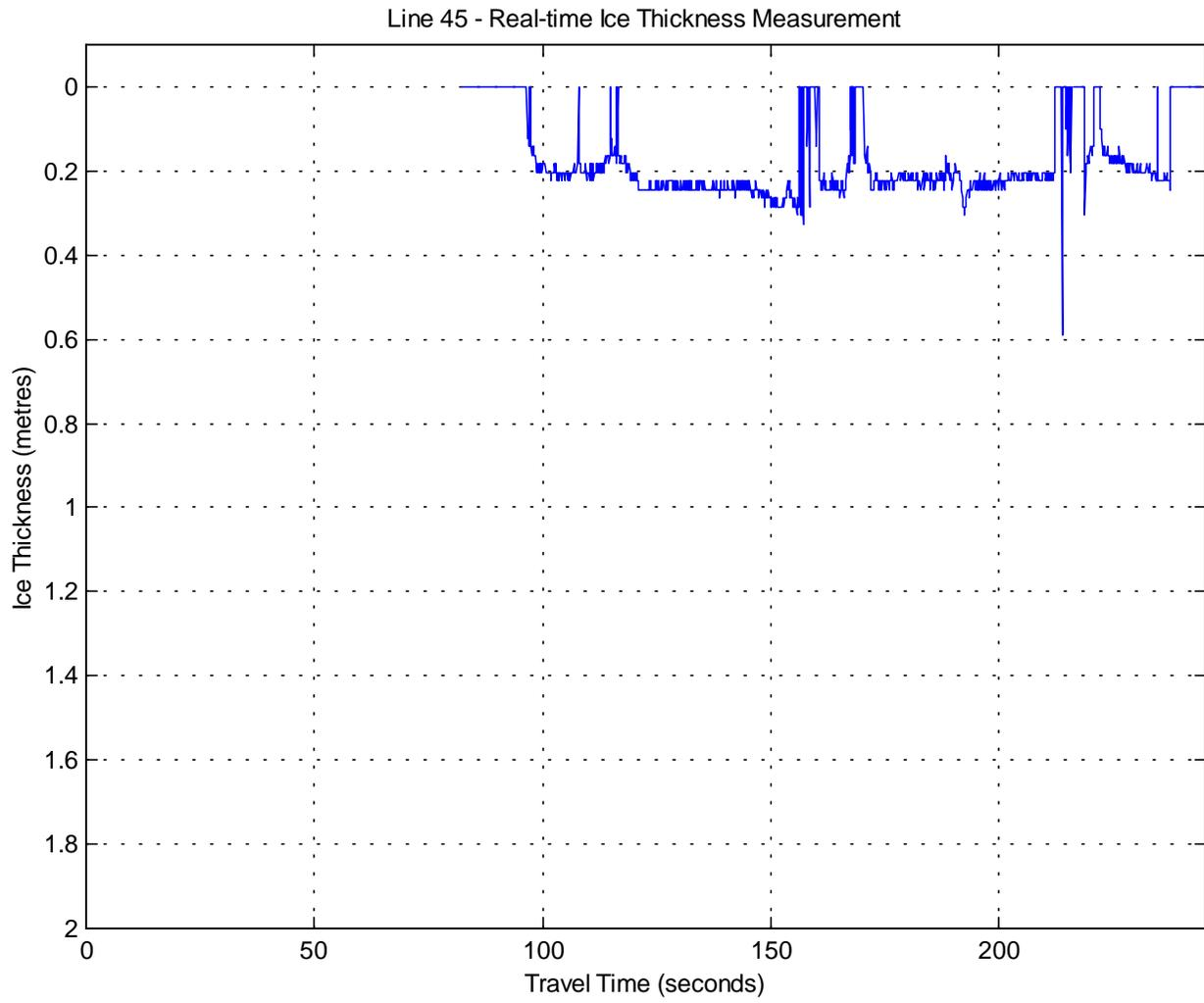
Figure 10. Plot of fresh water ice thickness measured with real-time system.
