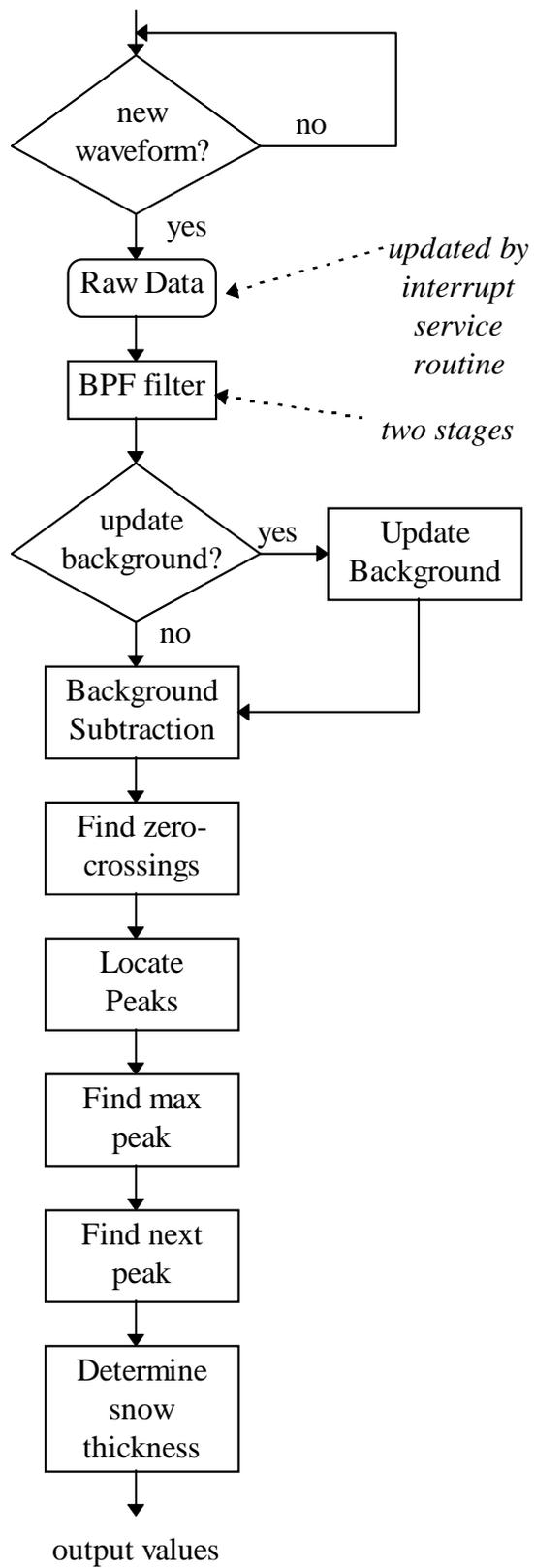
Figure 3. Block diagrams of the DSP software.
