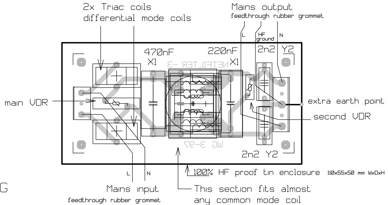
MULTIPURPOSE MAINS FILTER AND HF ISOLATION BOARD
