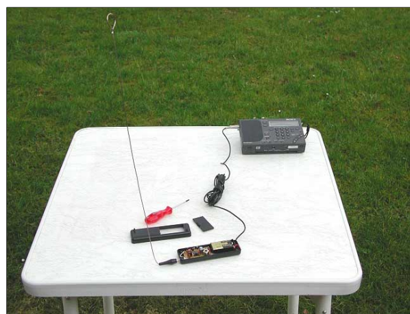
Figure 2. The circuit built on perforated board, and a setup with the SW1000.
