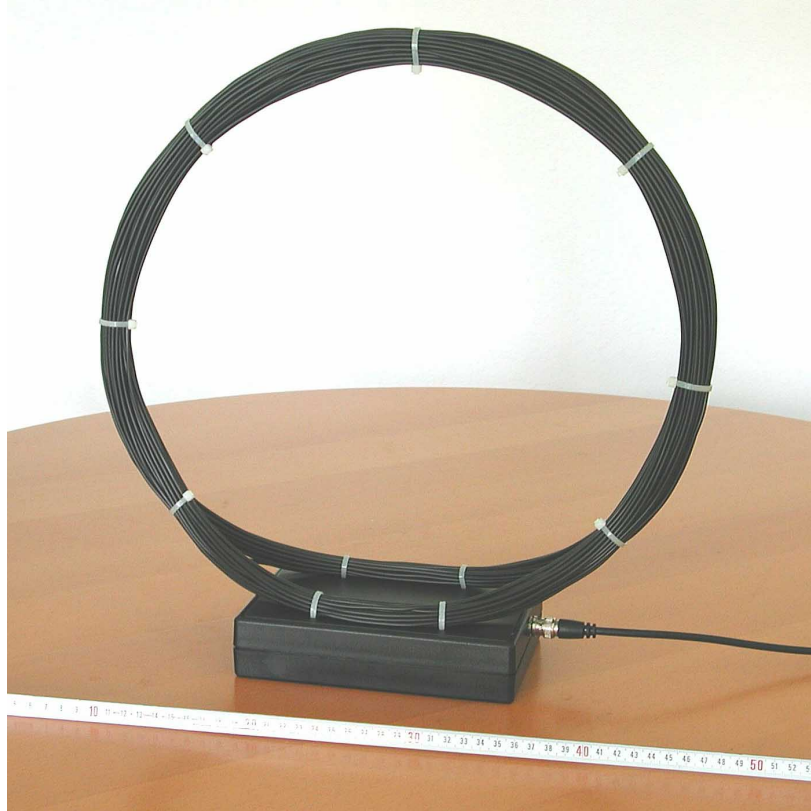
Figure 1. The prototype loop has 40 turns and a diameter of about 38 cm.
