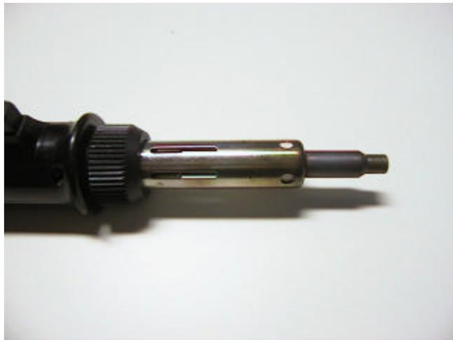
Fig 8 - Hot air tip on a Pyropen
