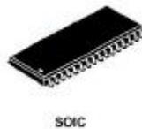
Fig 2 - Common SOIC package
