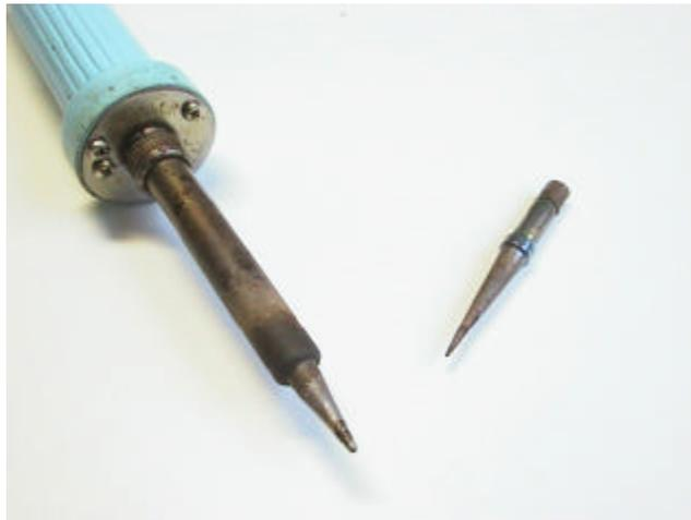
Fig 3 - Soldering Iron and Tip suitable for SMT
