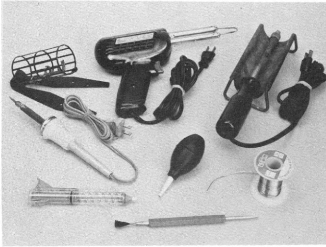
Fig. 1 — In this photo (l-r) are a pencil-type iron with stand, a soldering gun, and a large iron with cradle. Near the bottom of the photo are a solder sucker, vacuum bulb, soldering tool and 60-40 solder.
