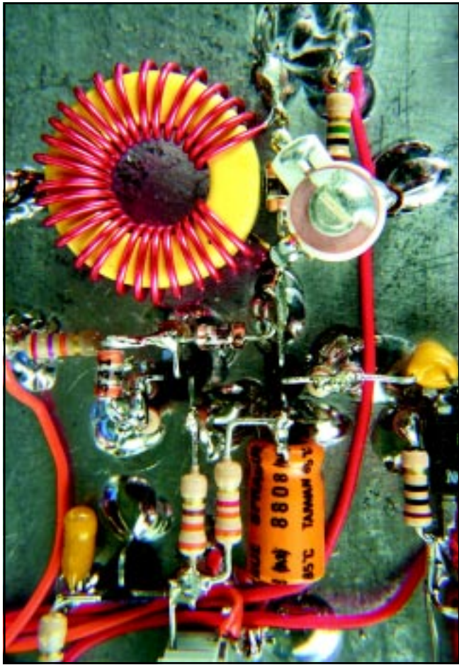
This ultra-tight close-up illustrates the so-called "dead-bug construction" that the author used in this version of the WBR. As an alternative, a circuit board is available from FAR circuits. 2
