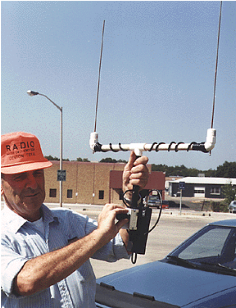
Jim Bryant, N5ZAV, uses this RDF antenna to get a bearing during a hidden transmitter hunt in Denton, Texas.
