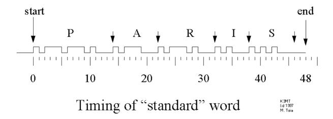
It starts at the "Start" mark. P has the pattern di dah dah dit. Look closely at the graph. Notice the structure of the dits and dahs, and the letter space after the last dit. A small arrow marks the end of P and the start of A. Follow the graph to see the structure of
