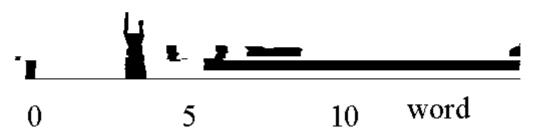
The "I" is "di dit" - two fast dits that, when you speak them, slur together, losing the "t" on all but the last dit. The "T" is a single dah. Notice the letter space between the I and T in the graph. Without it, the dits and dah will run together, making something not intelligible as "IT." The letter spaces are shown in bolder line width here only to emphasize that they are necessary parts of good Morse!
