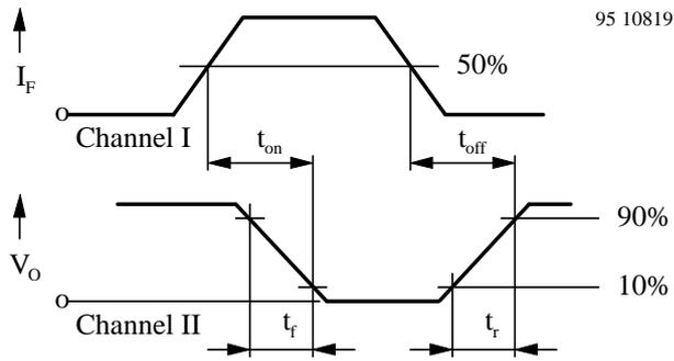
Figure 2. Pulse diagram
