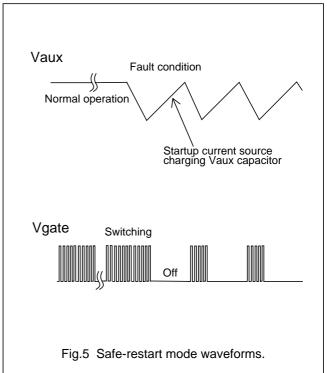
The startup current source also plays a key role in implementation of burst mode stand-by (see Irestart-stdby in Chapter "Characteristics"), which will be explained later.
