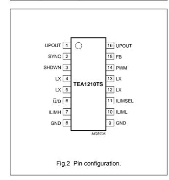
For all possible applications, the following groups of pins must be connected together:
