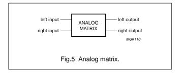
All switches and matrices are controlled via the I<sup>2</sup>C-bus.
