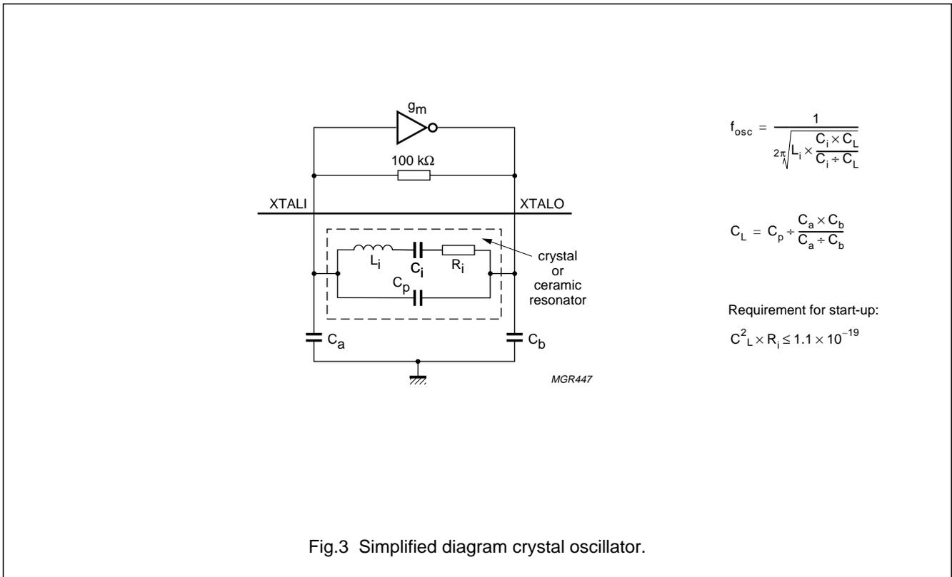
Fig.3 Simplified diagram crystal oscillator.
