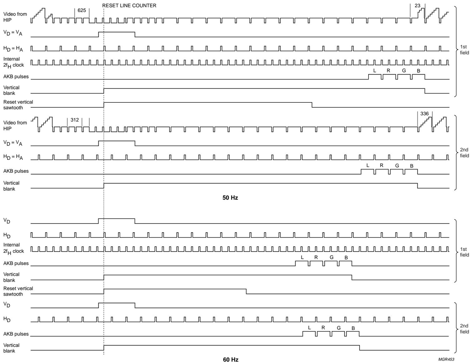
Fig.9 Vertical timing pulses for 1f<sub>H</sub> TV mode.
