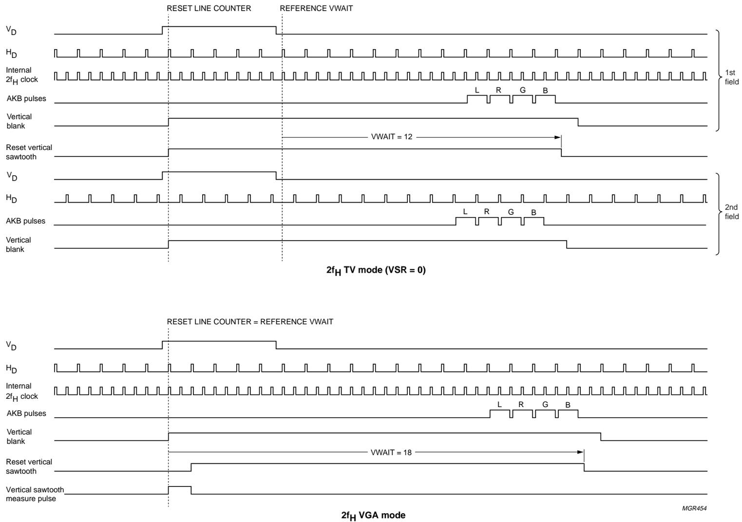
Fig.10 Vertical timing pulses for 2f<sub>H</sub> TV mode and VGA mode.
