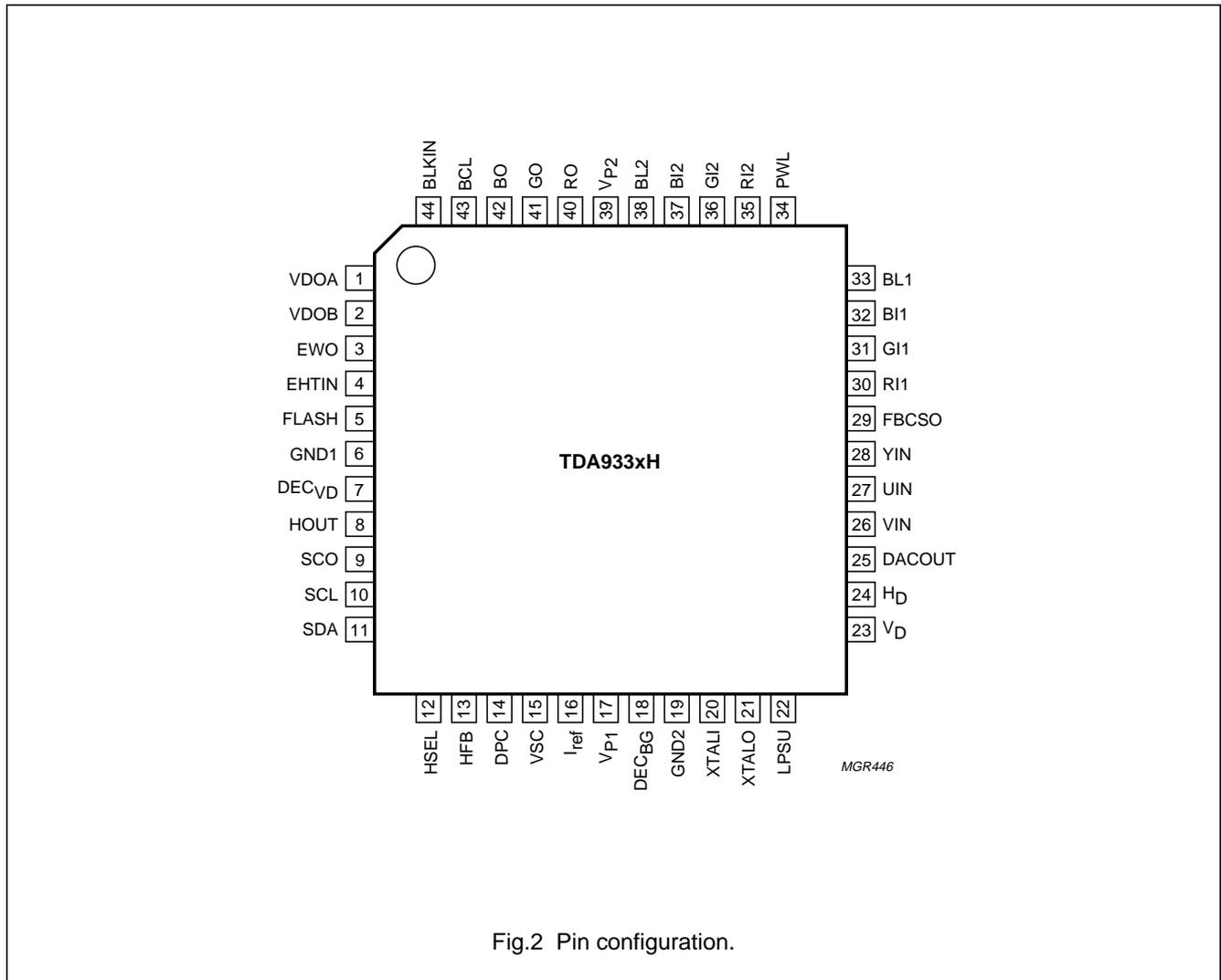
Fig.2 Pin configuration.
