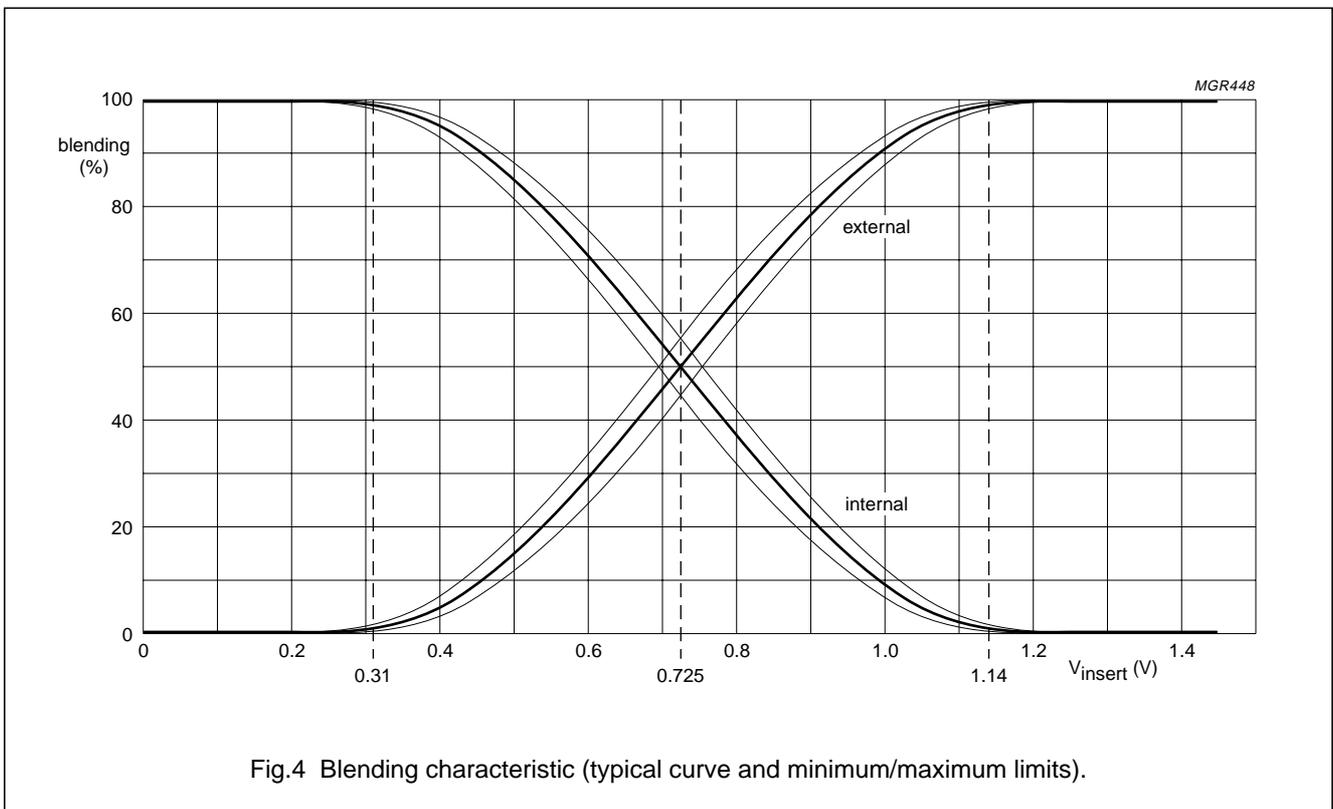
Fig.4 Blending characteristic (typical curve and minimum/maximum limits).
