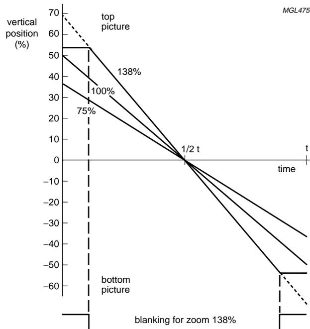
Fig.12 Vertical drive waveform and blanking pulse for different zoom factors.
