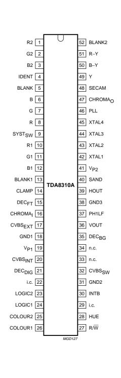
Fig.2 Pin configuration.
