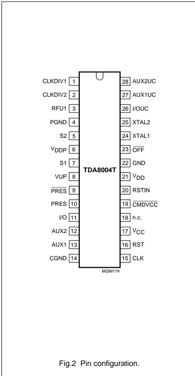
Fig.2 Pin configuration.
