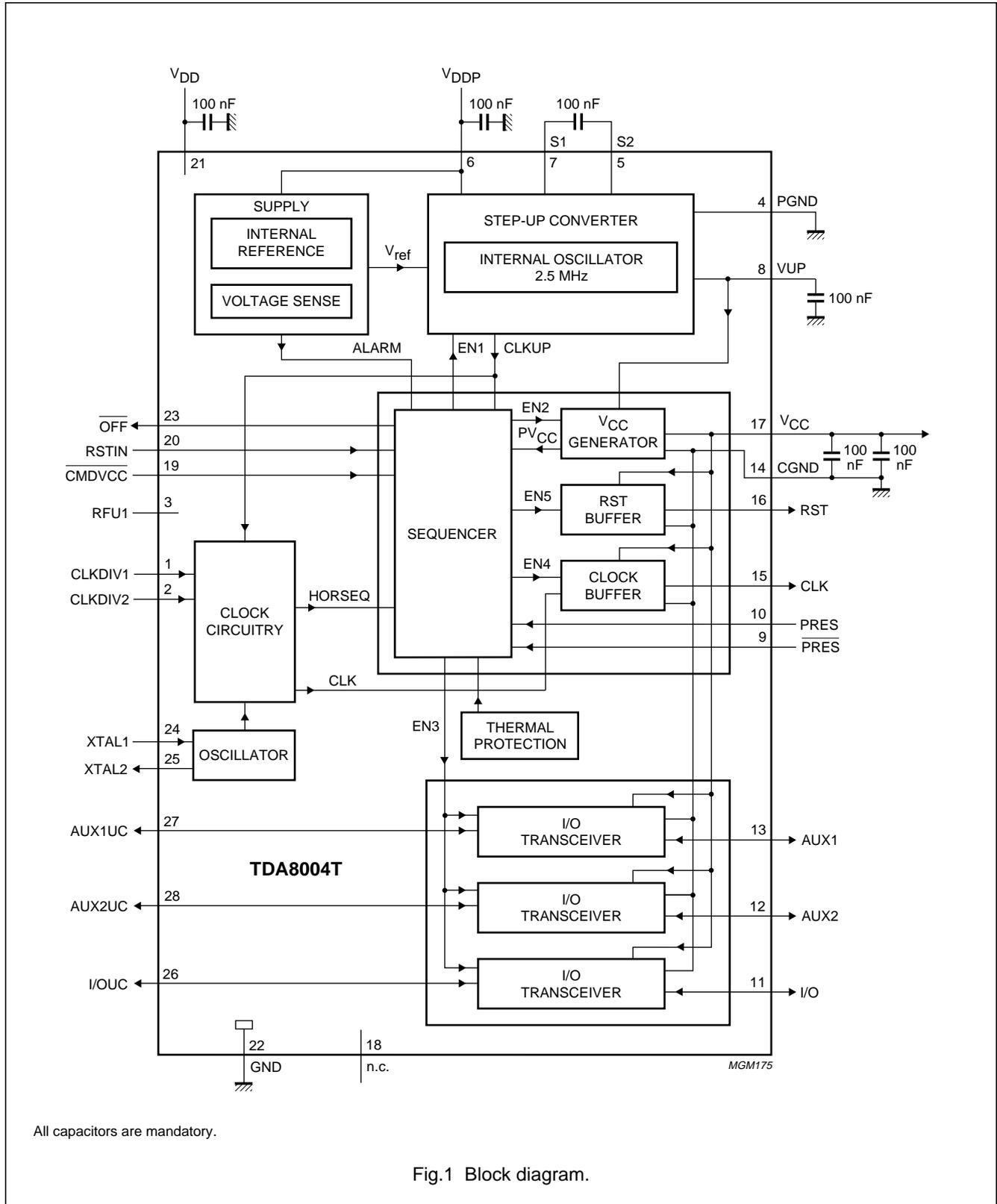
Fig.1 Block diagram.
