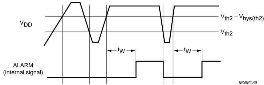
Fig.3 Alarm as a function of  $V_{DD}$  ( $t_W = 10$  ms).
