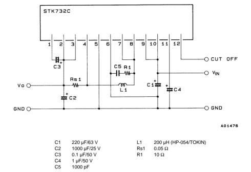
Note: Since pin 5 is grounded to the substrate, the noise level and other characteristics may be adversely affected if the heat sink is connected to the FG or GND lines. If this is a problem either make the heat sink floating or use an insulating sheet.
