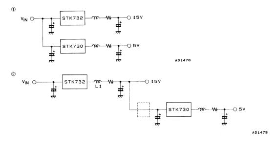
Note: It is possible for STK730 input ripple currents to cause L1 to vibrate audibly and adversely influence the 15 V system. If such problems occur, an inductor can be inserted at the point marked with dotted lines in the figure to form an LC filter.
