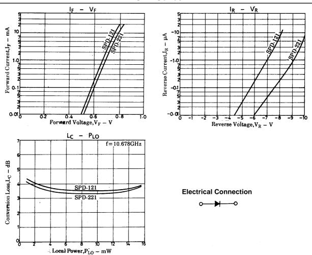
Note: In addition to the single types shown above, the integrated types shown below are available. For details, contact our sales offices.
