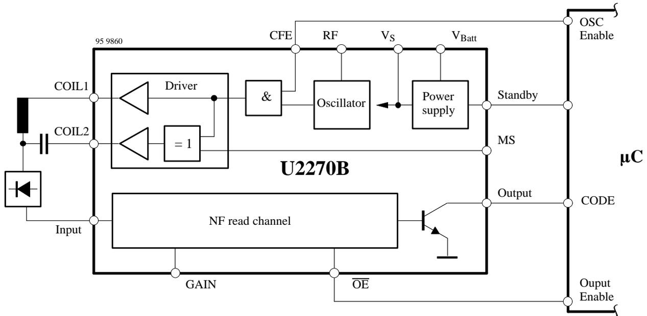
The U2270B serves as interface between the transponder and the microcontroller that compares the received data. This interface operates bidirectional.
