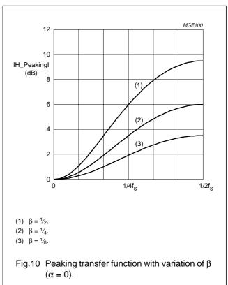
To compensate for a non-linear phase characteristic before the A/D converter, this filter will compensate such behaviour with a pulse response of  $[-\lambda, 1 + \lambda]$ .  $\lambda$  can be programmed for the values 0,  $\frac{1}{8}$ ,  $\frac{1}{4}$  and  $\frac{1}{2}$ .
