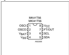
Figure 2B. SOIC Pin Connections
