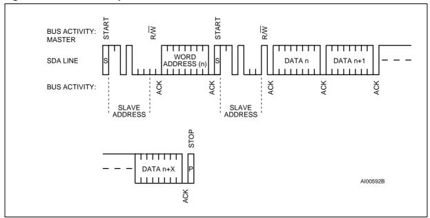
Figure 12. Alternate Read Mode Sequence
