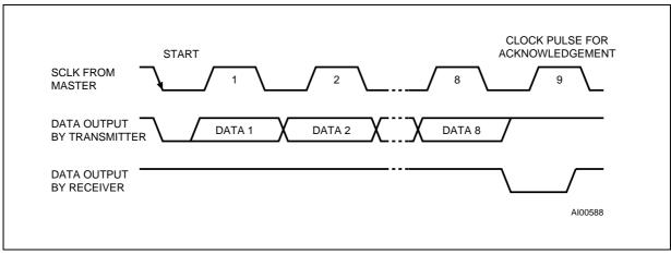
Figure 8. Bus Timing Requirements Sequence
