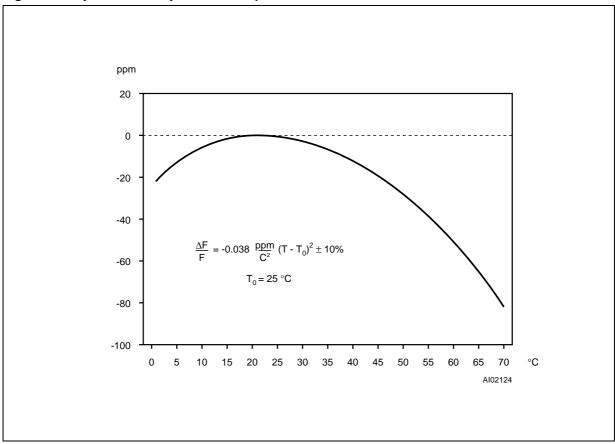
Figure 14. Crystal Accuracy Across Temperature
