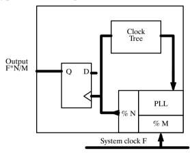
The maximum frequency at the PLL input after division by M is 70 MHz.
