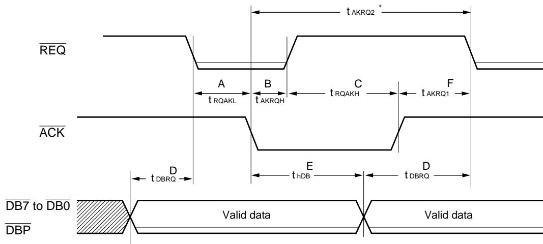
\*: The ACK "L" → REQ "L" time ( $t_{AKRQ2}$ ) is defined by either longer of ( $t_{AKRQH} + t_{RQAKH} + t_{AKRQ1}$ ) or ( $t_{hDB} + t_{DBRQ}$ ).
