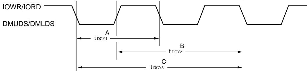
(b) Data register access cycle time (16 bit)
