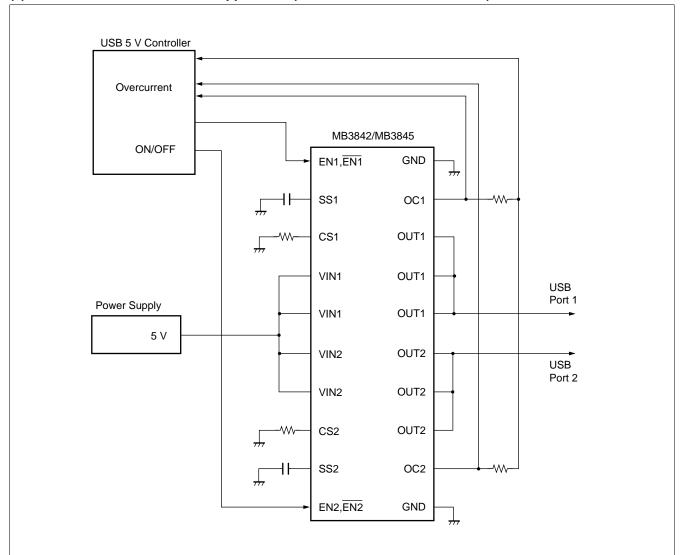
\*The MB3842 can also be adapted for use with 3.3V controllers.
