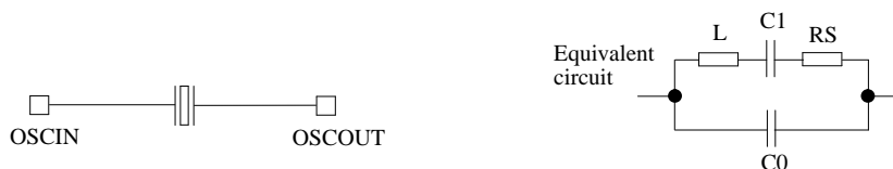
Figure 45. Crystal equivalent circuit
