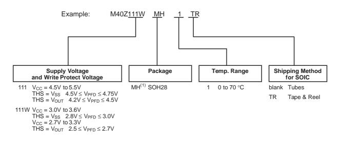
Note: 1. The SOIC package (SOH28) requires the battery package (SNAPHAT) which is ordered separately under the part number "M4ZxxBR00SH1" in plastic tube or "M4Zxx-BR00SH1TR" in Tape & Reel form.
