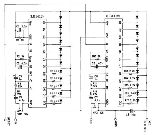
Note: Input signal of approximately 110 mVrms causes D8 (0 dB display) to light.
