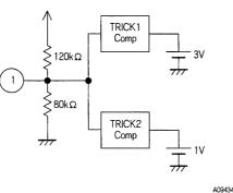
GND < pin 1 level - DC < 1.0 V: TRICK2 1.0 V < pin 1 level - DC < 3.0 V: NORMAL 3.0 V < pin 1 level - DC < 5.0 V: TRICK1
