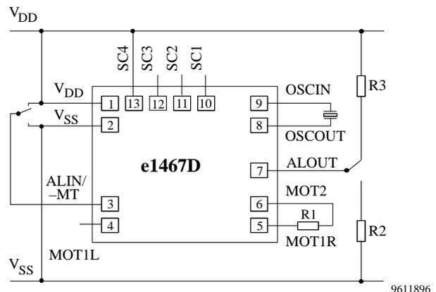
Figure 1. Functional test
