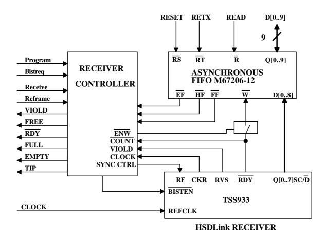
The HSDLink serial receiver must synchronize itself with the proper word alignment of the incoming data. Assertion of the HSDLink RF (ReFrame) input forces HSDLink to synchronize its internal bit counter with the boundary of a received K28.5 (SYNC) character. HSDLink will answer by asserting RDY low when the first K28.5 is received in the incoming flow. The receiver state machine controller should be designed to synchronize HSDLink at the beginning of data reception.
