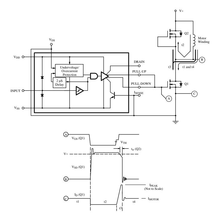
Figure 2. Clamping Inductive Flyback Energy
