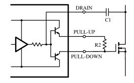
**Figure 6.** Simplified dv/dt Feedback Circuit
