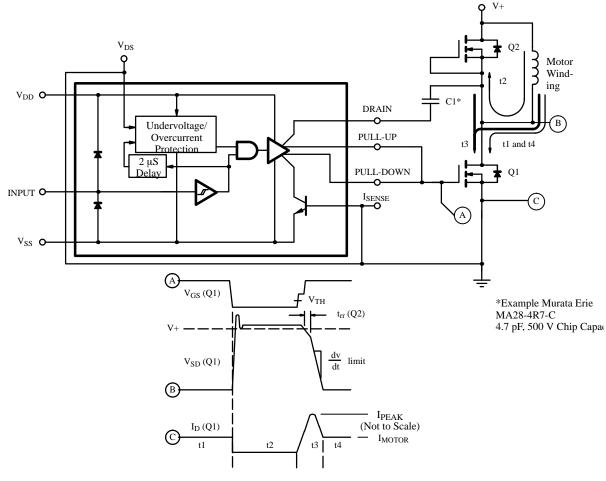
Figure 7. Direct dv/dt Limiting
