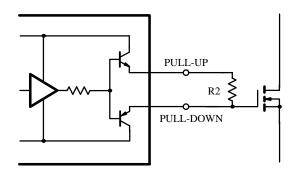
Figure 3a. Simplified "Split" Emitter-Follower Output Circuit
