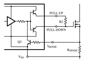
Figure 5. "Simplified Peak Shoot-Through Current Limiting Circuit
