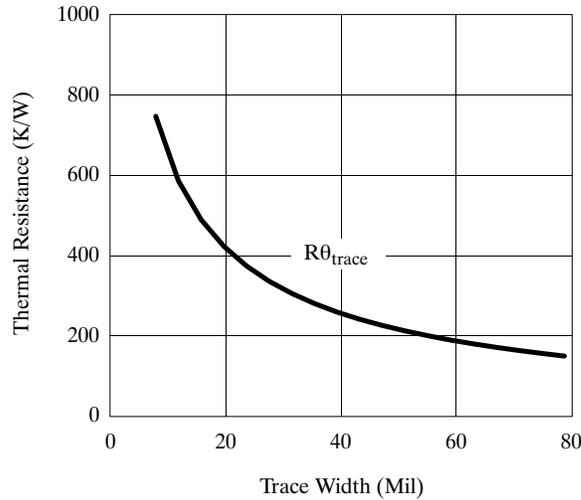
**Figure 7.** Trace thermal resistance vs. trace width
