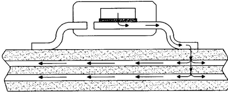
**Figure 3.** Thermal path with four-layer PCB
