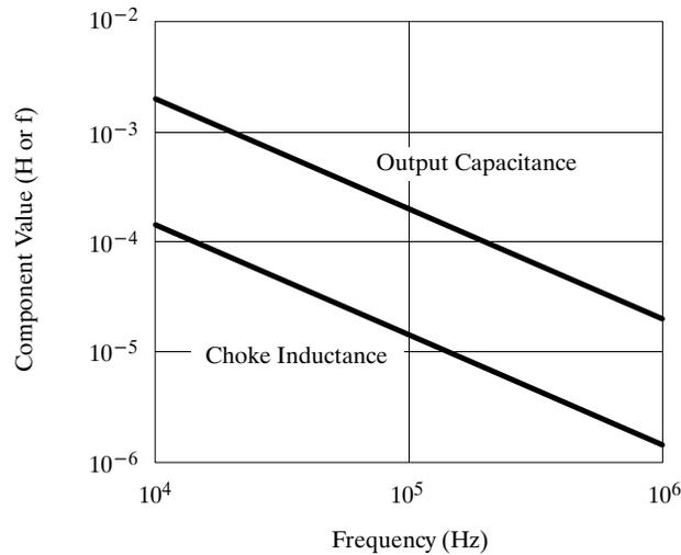
**Figure 1.** Output capacitance and choke inductance vs. frequency
