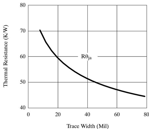
**Figure 8.** LITTLE FOOT thermal resistance vs. trace width
