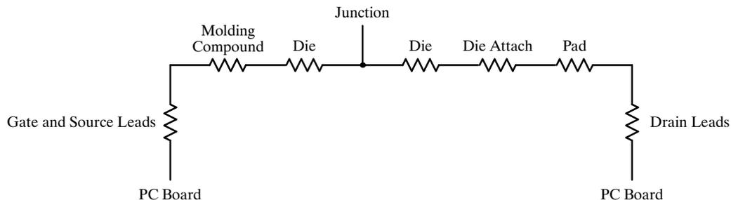
Figure 5. Power MOSFET thermal model
