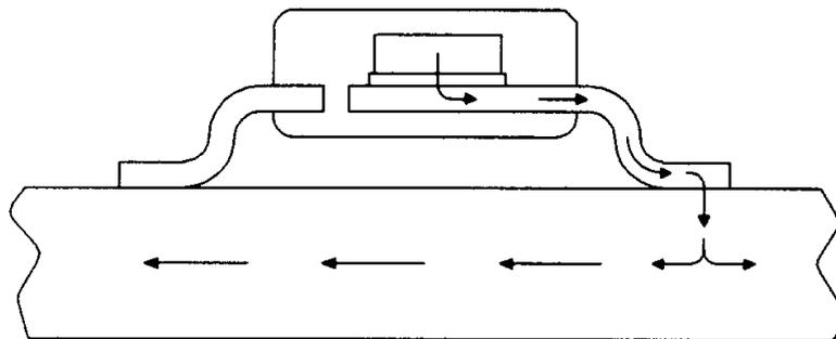
Figure 2. Thermal path in board-mounted power MOSFET
