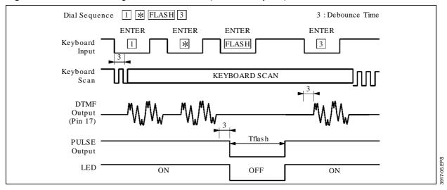
Figure 4: Pulse Mode Timing with Lighted Dial LED (Pin 24 to V<sub>DD</sub> or GND)
