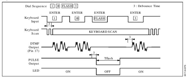
Figure 3: Tone Mode Timing with Tone Indicator (Pin 24 to any row)
