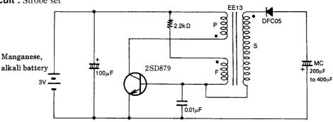
Core : EE13 (Kijima Wireless) Number of turns specified for transformer  $~P:0.55~\phi\times10~3/_{4}T,~S:0.07~\phi\times1350T$   $~F:0.23~\phi\times12~3/_{4}T$
