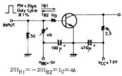
(For PNP, the polarity is reversed) Unit (resistance :  $\Omega$ , capacitance : F)
