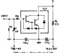
$PW = 50\mu s$ , Duty Cycle  $\leq 1\%$   $500I_B1 = -500I_B2 = I_C = 4A$ (For PNP, the polarity is eversed.) Unit (resistance:  $\Omega$ , capacitance: F)
