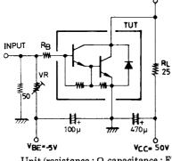
Unit (resistance :  $\Omega$ , capacitance : F) (For PNP, the polarity is reversed.)  $PW = 50\mu s$ , Duty Cycle  $\leq 1\%$
