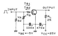
$\begin{array}{c} I_C \!=\! 10I_B1 \!=\! -10I_B2 \!=\! 1A & \text{Access} \\ \text{Unit (resistance : } \Omega, \text{ capacitance : } F) \end{array}$
