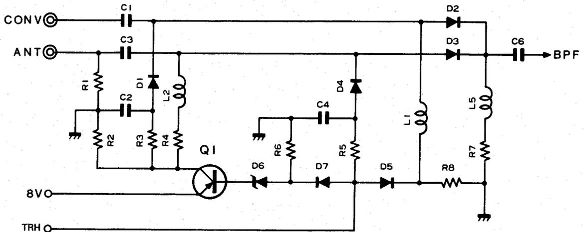
The signal (1.6 ~ 30 MHz) received from the antenna connector (ANT2) is fed to the input selecting circuit.
