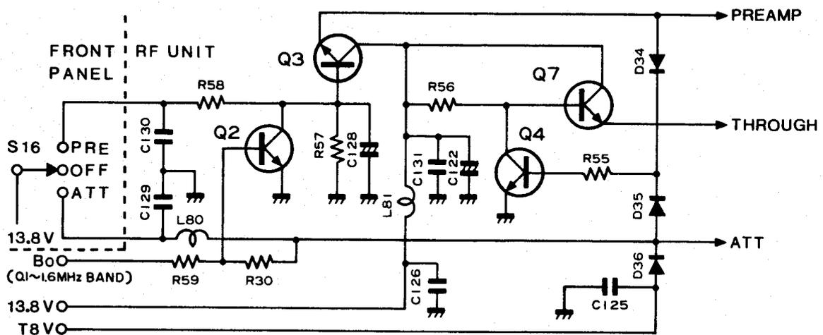
When the OFF position is selected, only Q7 is turned ON, and voltage is supplied to the through circuit. When PREAMP is selected, the 13.8V from the PRE/ATT switch is divided at R57 and R58, is applied to the Q3 base, Q3 is turned ON, and the preamplifier circuit which employs push-pull of junction-type FETs Q5 and Q6 operates.
