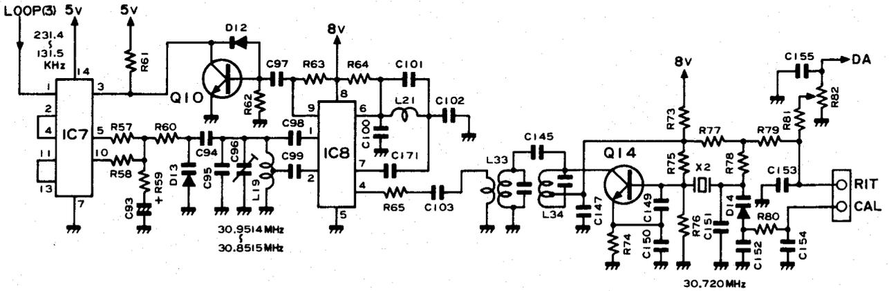
IC7 is a phase comparator; the reference frequency (131.5 ~ 231.4 kHz) divided to 1/100 the 3rd loop output by IC5 is applied to pin 1.
