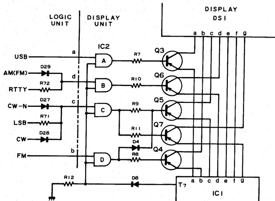
The four AND gates (IC2A ~ D) are controlled by the timing signals (a ~ d) from the logic unit and  $T_7$  of IC1.
