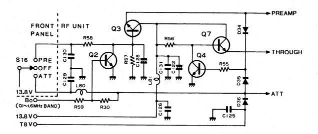
When the OFF position is selected, only Q7 is turned ON, and voltage is supplied to the through circuit. When PREAMP is selected, the 13.8V from the PRE/ATT switch is divided at R57 and R58, is applied to the Q3 base, Q3 is turned ON, and the preamplifier circuit which employs push-pull of junction-type FETs Q5 and Q6 operates.
