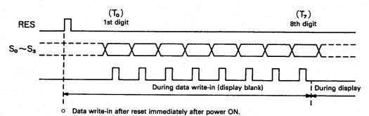
There is no necessity for reset when writing in data second time and thereafter. When the first pulse of CTL input is input, the display is blanked; when the eighth pulse is input and the write-in is input, the display starts again.
