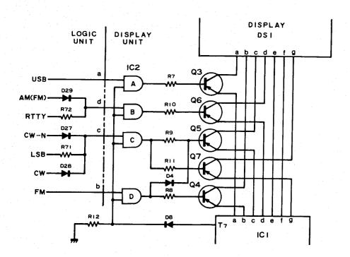
The four AND gates (IC2A  $\sim$  D) are controlled by the timing signals (a  $\sim$  d) from the logic unit and T<sub>7</sub> of IC1.
