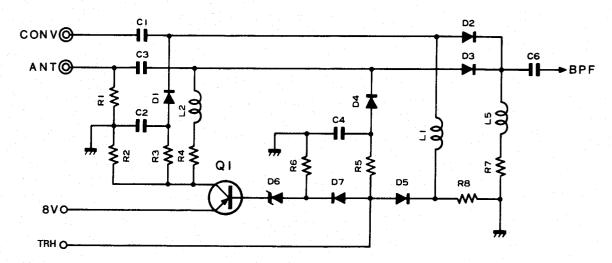
The signal (1.6  $\sim$  30 MHz) received from the antenna connector (ANT2) is fed to the input selecting circuit.
