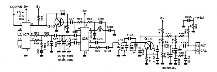
IC7 is a phase comparator; the reference frequency (131.5  $\sim$  231.4 kHz) divided to 1/100 the 3rd loop output by IC5 is applied to pin 1.
