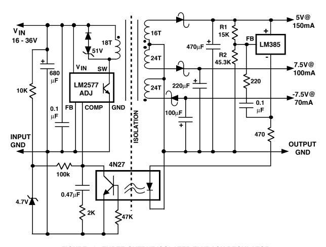
FIGURE 52. THREE-OUTPUT ISOLATED FLYBACK REGULATOR
