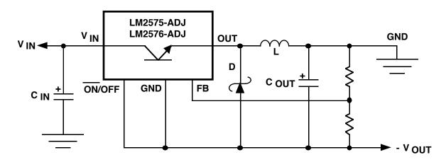
FIGURE 54. LM2575 AND LM2576 INVERTING APPLICATION
