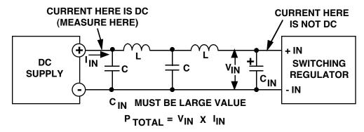
FIGURE 47. L-C FILTER USED IN DC INPUT CURRENT MEASUREMENT
