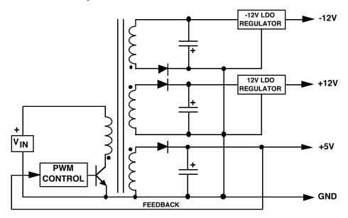
FIGURE 34. TYPICAL MULTIPLE-OUTPUT FLYBACK
