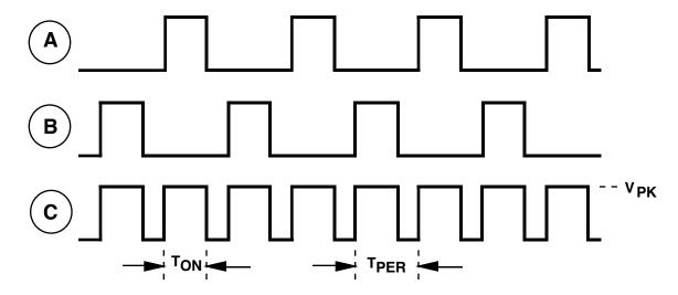
FIGURE 36. TIMING DIAGRAM FOR PUSH-PULL CONVERTER
