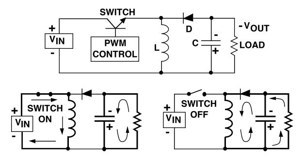
FIGURE 32. BUCK-BOOST (INVERTING) REGULATOR
