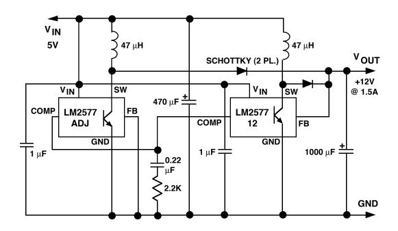
FIGURE 50. DUAL LM2577 BOOST CIRCUIT
