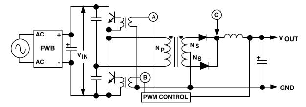
FIGURE 37. HALF-BRIDGE CONVERTER
