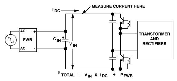
FIGURE 48. MEASURING INPUT POWER IN OFF-LINE CONVERTER
