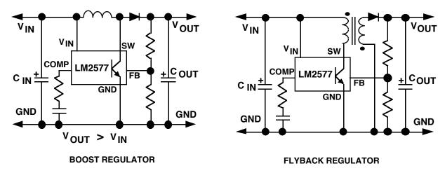
FIGURE 49. BASIC APPLICATION CIRCUITS FOR THE LM2577
