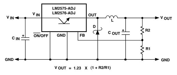
FIGURE 53. LM2575 AND LM2576 BUCK REGULATOR APPLICATION
