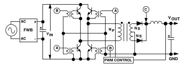
FIGURE 39. FULL BRIDGE CONVERTER
