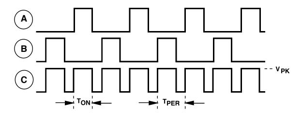
FIGURE 38. TIMING DIAGRAM FOR HALF-BRIDGE CONVERTER
