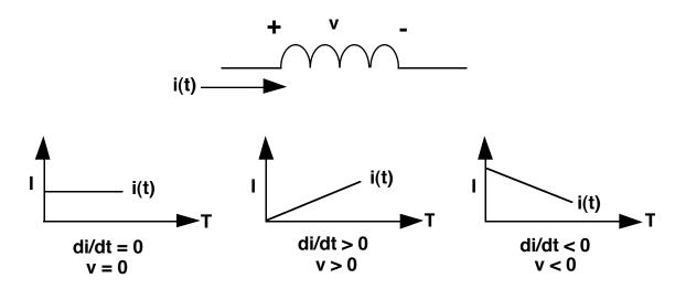
FIGURE 25. INDUCTOR VOLTAGE/CURRENT RELATIONSHIP
