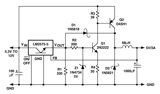
FIGURE 55. LOW-DROPOUT 5V/3A REGULATOR
