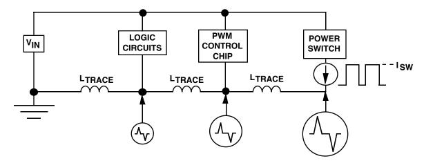
FIGURE 41. EXAMPLE OF POOR GROUNDING
