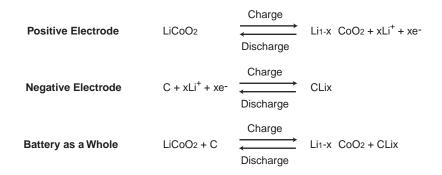
The principle behind the chemical reaction in the lithium ion battery is one where the lithium in the positive electrode lithium cobalt oxide material is ionized during charge, and moves from layer to layer in the negative electrode. During discharge, the ions move to the positive electrode and return to the original compound.
