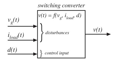
Load current variations: a significant step-change in load current, such as from 50% to 100% of rated value, may be applied.
